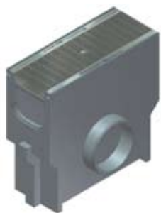
Trash box with galvanised bucket, with mesh grating MW 30/10, galvanised, class B 125, locked
